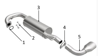
(Carefully read all instructions before installation) Disconnect the vehicle's battery before removal of the OEM exhaust system. This will prevent electrical accidents and will reset the computer if it applies to the vehicle. Remove existing exhaust system from the vehicle. Only remove parts that will be replaced. Clean existing flange with a wire brush to ensure proper sealing.
